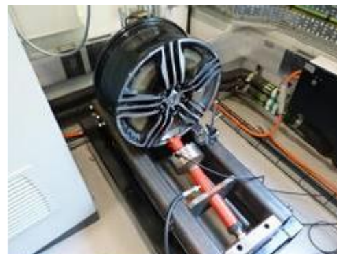
Application of lateral loads to represent cornering forces
