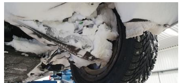
Snow packing around the IWM during winter vehicle testing
