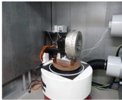
Shock and vibration testing is conducted at levels between two and four times greater than centralised drivetrains
