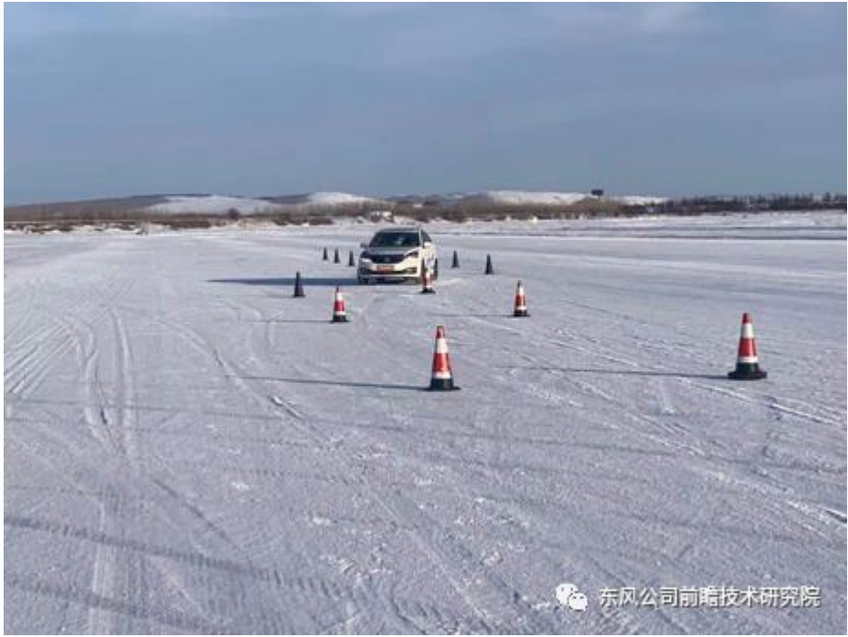
Speed 77km/h through double shift line
