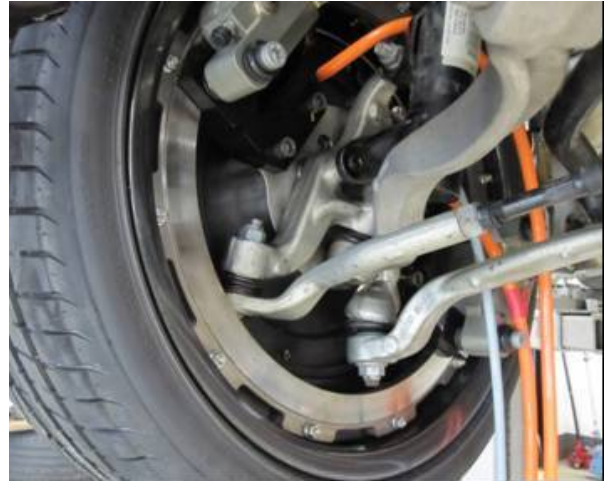
Figure 9: Right motor and brake assembly with wheel
