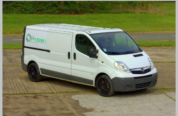
Available at HTUF for ride requests is the Vivaro diesel hybrid. Protean Electric and Millbrook Proving Ground, one of Europe’s leading vehicle test and demonstration centers, partnered to produce the Vivaro diesel hybrid. With the Protean conversion kit of two Protean Electric PD-18 motors attached to the rear axle, the two motors together provide torque assist of up to 1,180 lb.-ft. (1,650 Nm) peak and 740 lb.-ft. (1,000 Nm) continuous at the rear wheels. Inquire at Protean booth 806.
