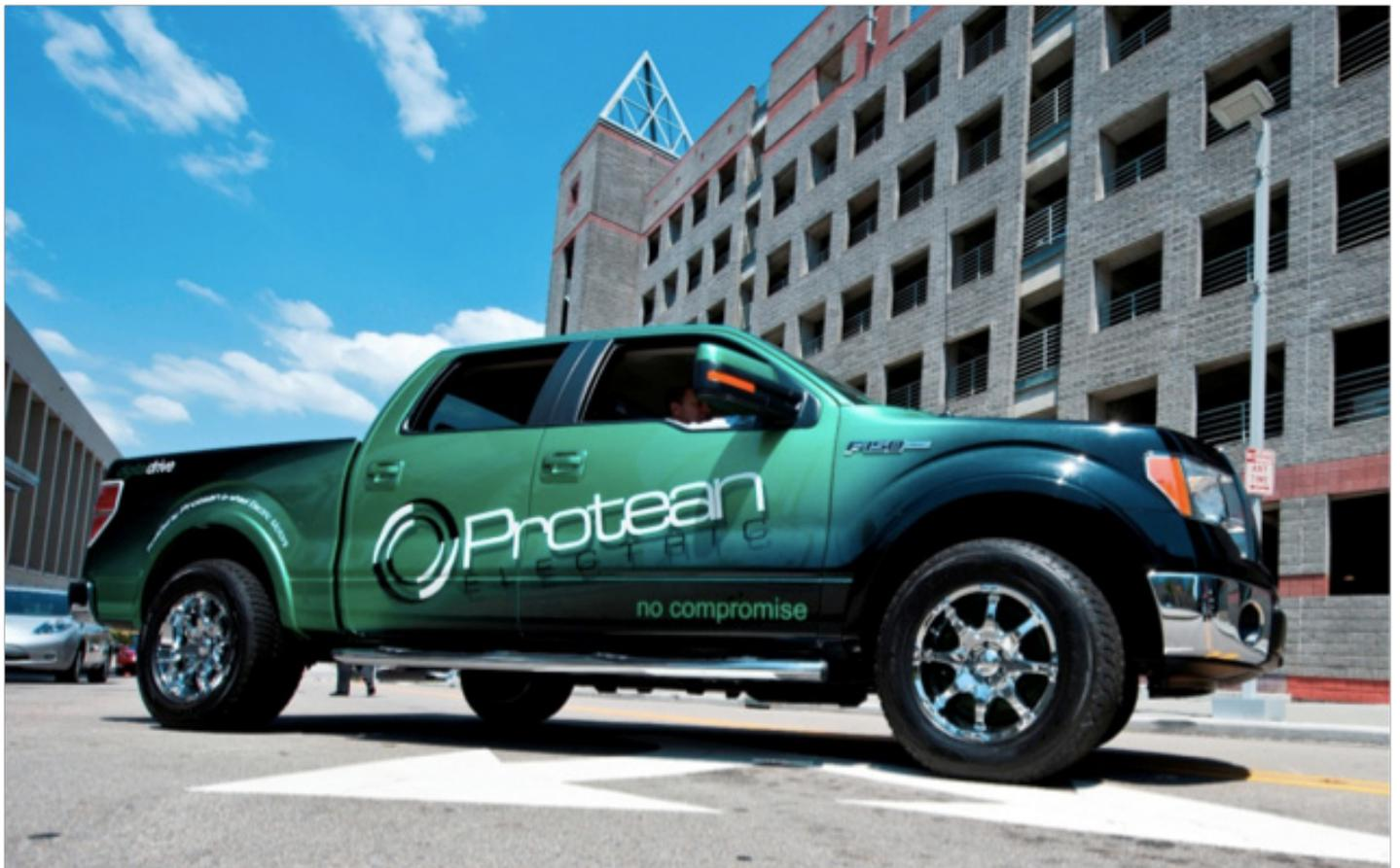
Protean’s fully electric Ford F150 pick-up demonstrates the benefits of the company’s in-wheel motors and ability to retrofit them on existing vehicles. Protean Electric added motors to each wheel, removed the conventional IC engine and installed a 40kWh battery, giving the truck an electric range of 100 miles. This vehicle will be on display in Protean’s booths 706 and 806.
